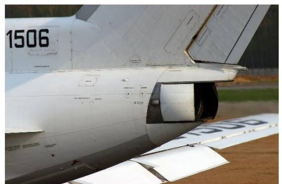
Bucket thrust reverser on the center engine
